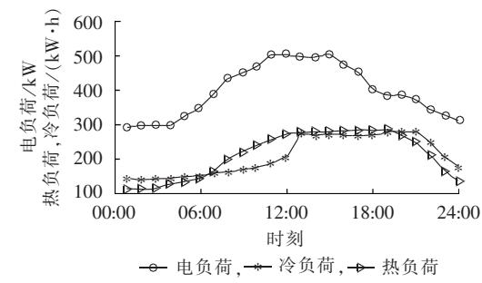
Fig.3 Typical daily cool,heat and power load curves
